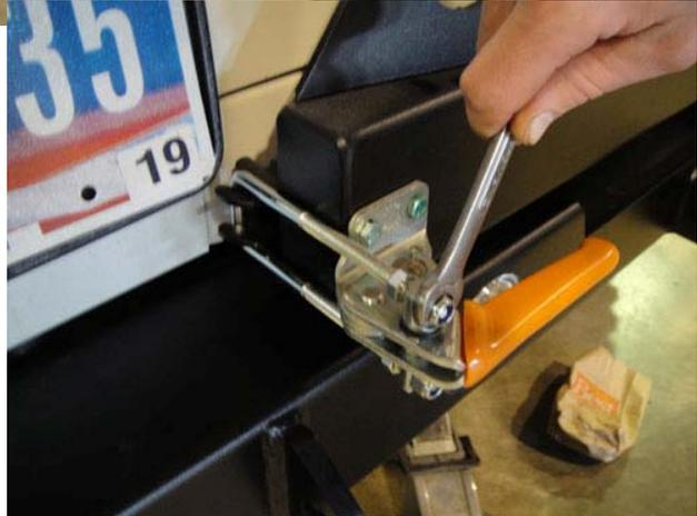
**21.** Next Install the L-Brackets shown with the Red arrow using the supplied 3/8" x 2.5" long bolts. The L bracket will make contact with the Rubber isolators on the back of your door shown by the yellow arrow. Unlatch the handle shown in the step above and adjust the L-Bracket to make tight contact with the rubber isolator and relatch the handle to make sure its tight.
