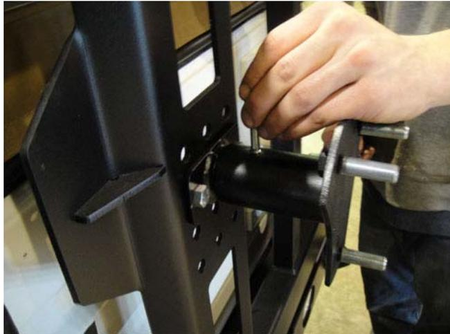
**25.** You will need to adjust the mount so when you tighten the lug nuts, the tire makes good tight contact with the tire carrier as shown. **DO NOT** mount the tire without it making contact with the tire carrier. This will cause rattles. Read below for more info.
