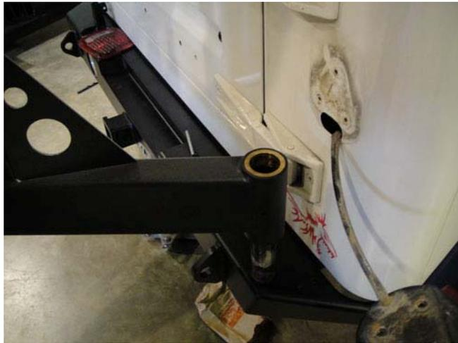
**17.** Install the grease zerk and gently snug in place. You can grease after everything is installed with a grease gun.
