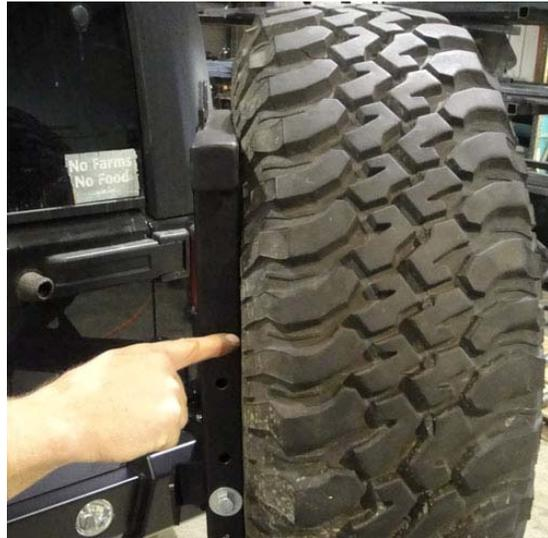
**26.** The pic below shows that the tire mount does not actually have to touch the back of the wheel. When installed. Most importantly the tire itself needs to be tight against the tire carrier frame as shown above.
