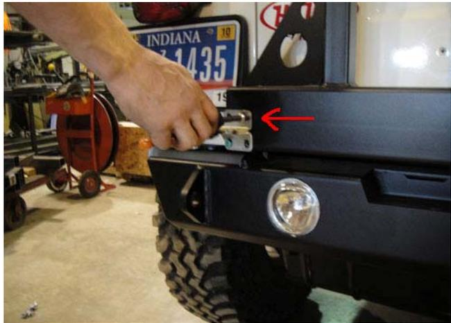
**20.** With the latch bolted in place, install the U bolt as shown and adjust. Latch and unlatch the handle and adjust as necessary to make sure the handle latches tightly.
