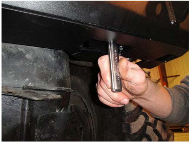
**13.** Next apply grease to the hinge pin. Smear a small amount all over the pin before installing the tire carrier.
