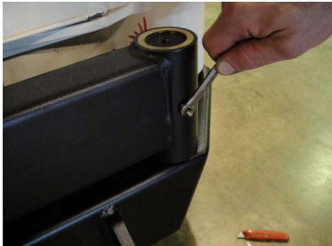
**18.** Next install the pin brace using 4 (3/8" x 1") bolts. Three of them will bolt into the bumper as shown by the blue arrow and 1 will thread into the Spindle as shown by the red arrow. NOTE: install a washer on top of the spindle between the spindle and pin brace as shown by the YELLOW arrow. This prevents the brace from contacting the carrier when it is rotated open and closed.
