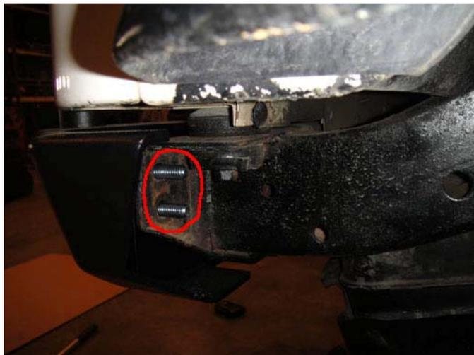
**11.** Next install the last 4 bolts using the mounting plates from step 7. Place the mounting plates up behind the cross-member.
