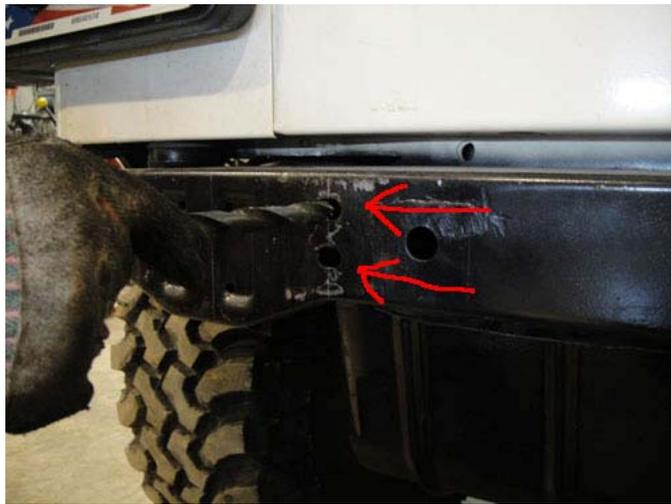
6. Install the reverse lights in the bumper. **Note:** The lights provided may differ from the ones pictured. Follow the instructions on back of the box that the lights came in for the wiring instructions.
