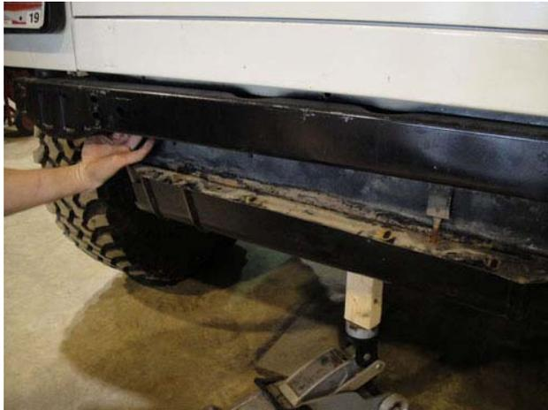
4. The widest set of holes on each side of the LoD bumper will match up to the existing holes of the rear cross-member. If you have a TJ or an Unlimited you will need to drill the two inside holes for each side.
