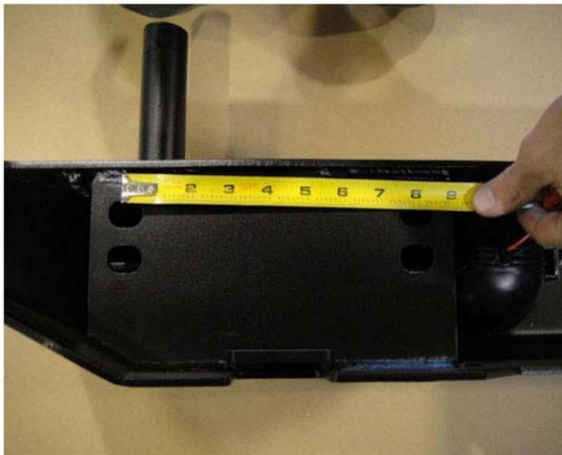
5. The picture here shows two of the holes that will need to be drilled if you have a TJ or Unlimited. Use a center punch to mark the exact location of the scribe marks from the previous step. When drilling be sure to use a small drill bit to pilot drill the holes first. Finish drilling these holes with a 1/2" drill bit. These four holes are all you need to drill to install this bumper.
