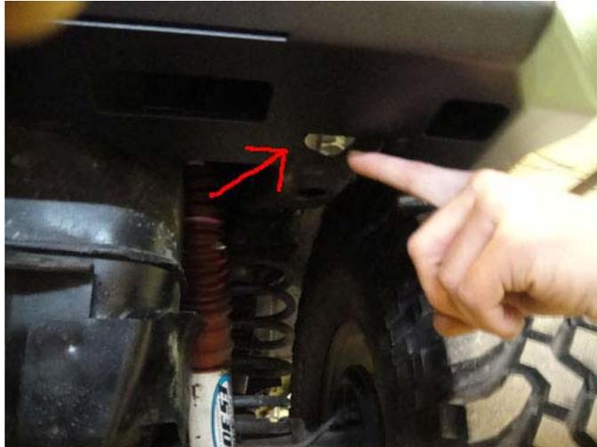
**9.** Next install the 4 bolts (7/16" x 1.50" ) on the outermost mounts of the bumper and crossmember. Install with a washer and 7/16" nut on each but do not tighten yet.
