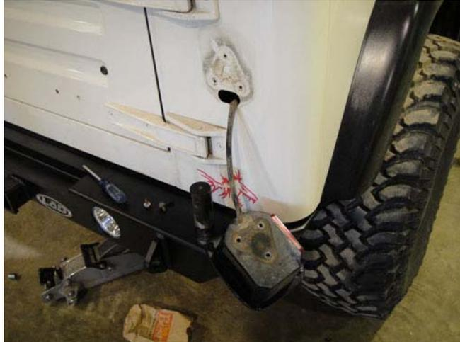
**16.** With the tail light removed slide the tire carrier down onto the hinge pin. **Note:** You may have to swing the carrier open and closed while pushing down at the hinge side. Be sure to support the latch end of the carrier while doing this to obtain the proper alignment to prevent the carrier from binding on the pin.
