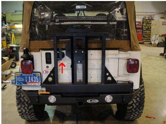
**24.** Next install the tire mount with the 3-1/2” studs. If you have the newer mount this piece will vary in looks also. The mount is adjustable for different backspaced wheels. Before you mount the tire read the steps below on how to choose the setting you need!
