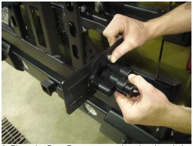
3. Place the Roto-Pax mount against the slotted plates. These mounts are also adjustable forward and back. This allows the cans to be mounted as close to the body as possible.
