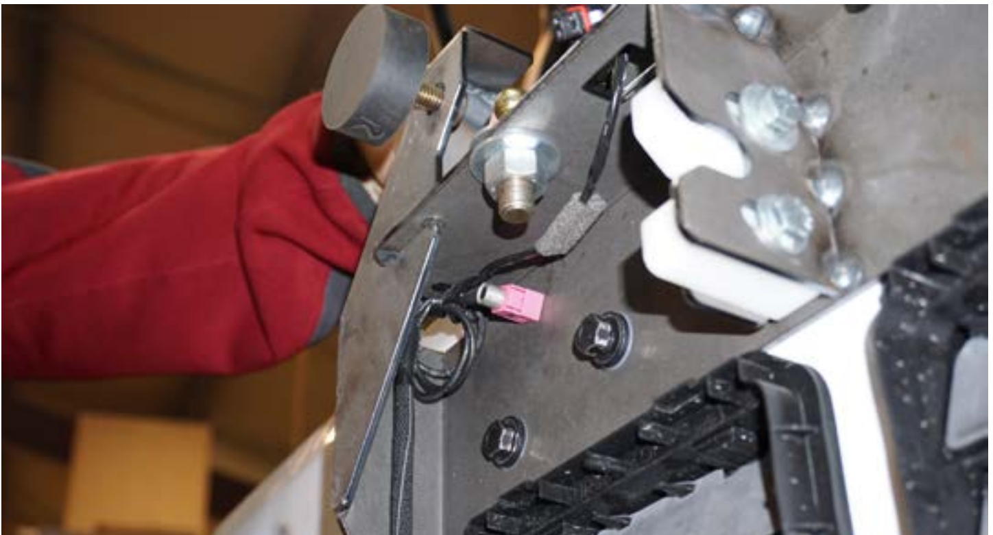
Tie up the old camera wire inside the door plate as shown. If you are running a third brake light, run it through the indicated hole. If not, also tie it up.
