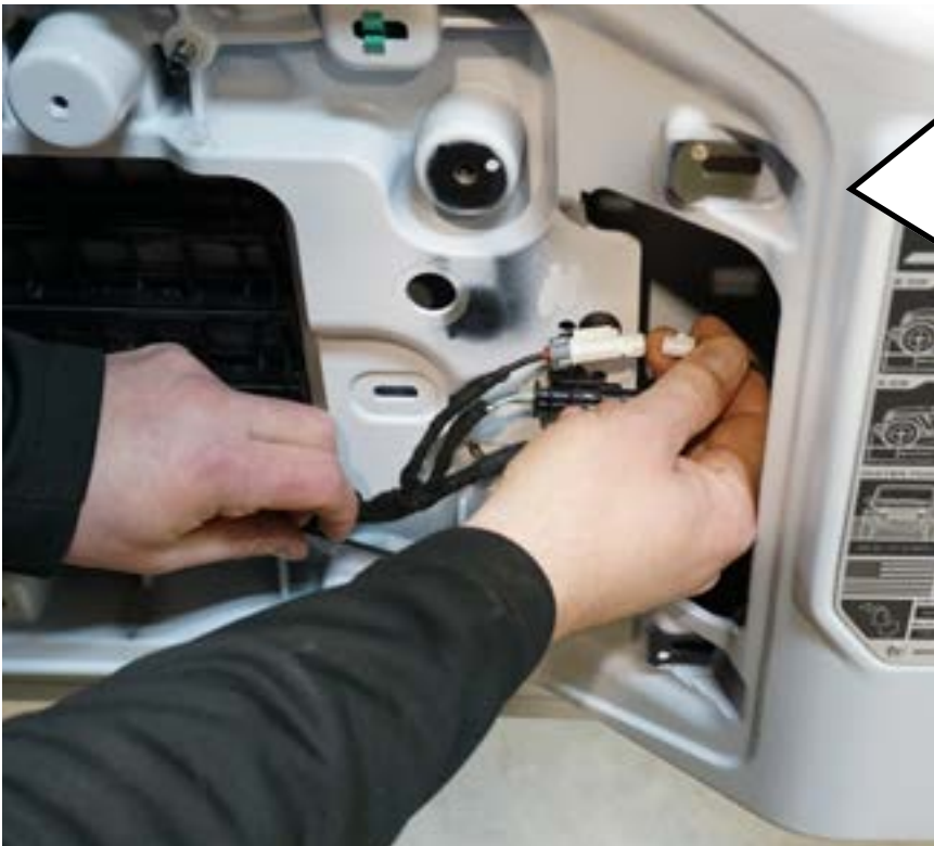
Plug the extension in, replace the grommet back into the hole.
