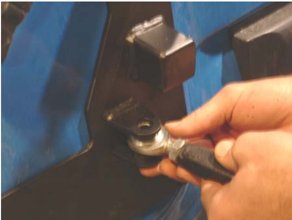
31. Place the adjustable link onto the plate located on the door. There will be (2) two spacers in the hardware kit that need to be placed on each side of the rod end. Place the tapered edge of each spacer in toward the rod end and tighten. Note: We recommend using Loctite on all the threads of the bolts and linkage arm to prevent them loosening or movement in the thread.
