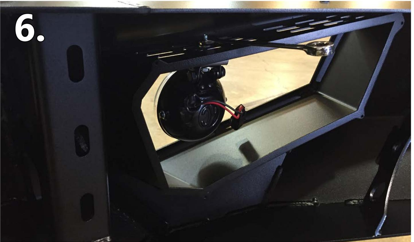
Before proceeding further, attach your lights into the holes. There are slots provided on the top face of the light opening.
