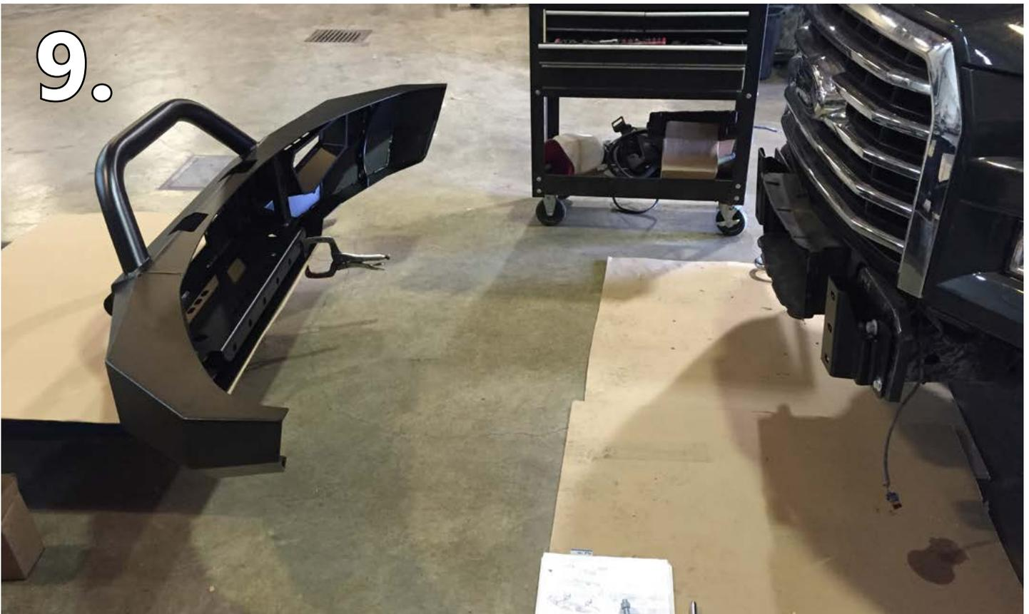
9. It helps to have something like a pallet jack during the install to hold the bumper up to the mounts while you attach it.
