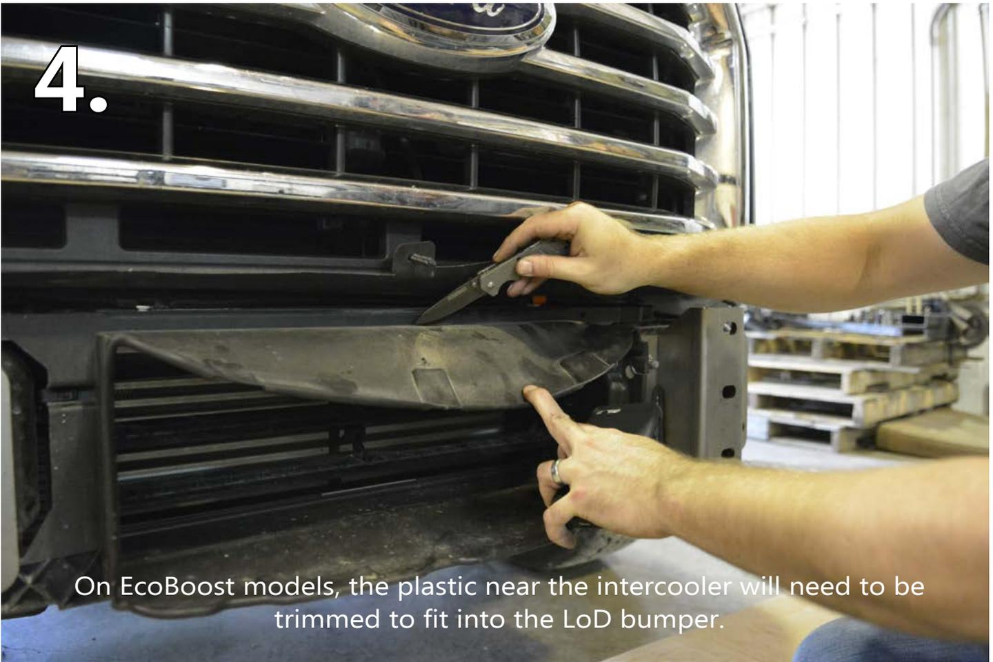
On EcoBoost models, the plastic near the intercooler will need to be trimmed to fit into the LoD bumper.
