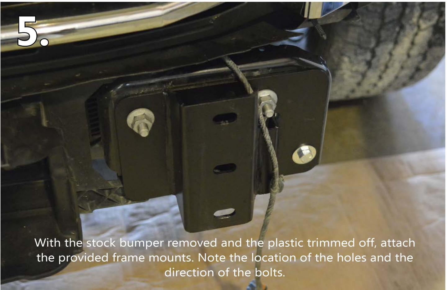
With the stock bumper removed and the plastic trimmed off, attach the provided frame mounts. Note the location of the holes and the direction of the bolts.
