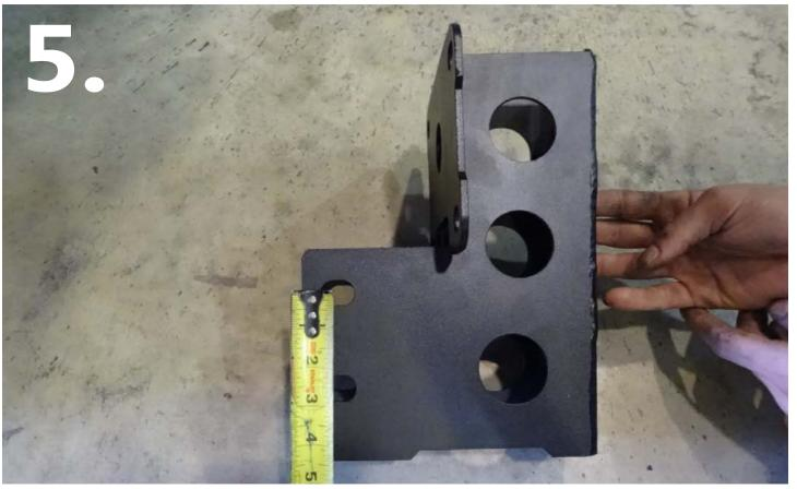
THE BACK HOLES ON THE MOUNTS WILL NEED THE FRAME DRILLED. THE HOLE SPACING FOR THESE HOLES (CENTER TO CENTER) WILL BE 2-1/2". THESE HOLES SHOULD BE DRILLED WITH A 9/16" DRILL BIT.
