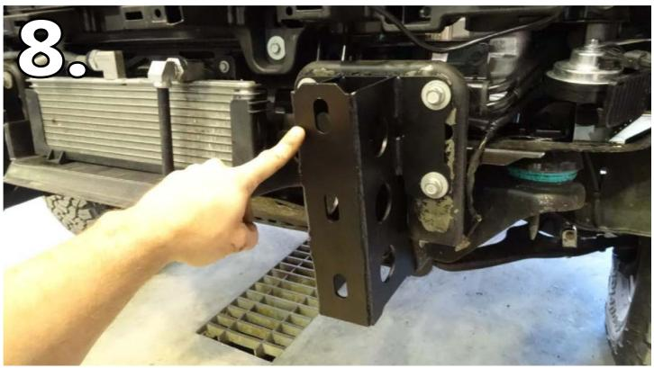
WITH THE FRAME MOUNTS INSTALLED, TIGHTEN ALL 8 OF THE **1/2**" x **1-3/4**" BOLTS. THE FRAME MOUNTS ARE SLOTTED IN DIFFERENT DIRECTIONS TO ALLOW ADJUSTABILITY WHEN MOUNTING THE BUMPER.
