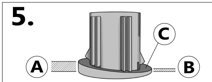
When positioning the sensors, also pay attention to the bezel. Side "A" is thicker than "B", to seat the sensor at an angle. You must position it in the same way as in the factory bumper. Apply a dab of glue to the surface labelled "C"
