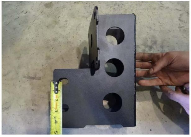
THE REAR HOLES ON THE MOUNTS WILL NEED TO HAVE THE FRAME DRILLED. THE HOLE SPACING FOR THESE HOLES (CENTER TO CENTER) WILL BE 2-1/2". THESE HOLES SHOULD BE DRILLED WITH A 9/16" DRILL BIT.
