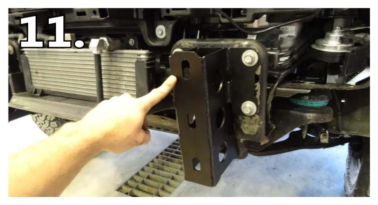
WITH THE FRAME MOUNTS INSTALLED, TIGHTEN ALL 8 OF THE **1/2**" x **1-3/4**" BOLTS. THE FRAME MOUNTS ARE SLOTTED IN DIFFERENT DIRECTIONS TO ALLOW ADJUSTABILITY WHEN MOUNTING THE BUMPER.
